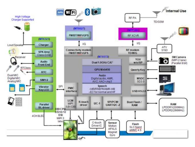
MT6572 functional system is made of three parts as below:
